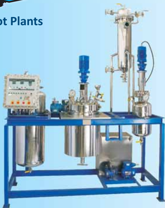
Ex-proof hydrogenation pilot plant with catalyst charging, catalyst filter with recycle & catch pot
