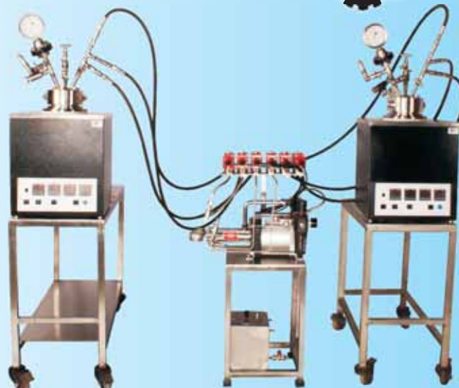
Bottom stirred with automatic pressure control system
