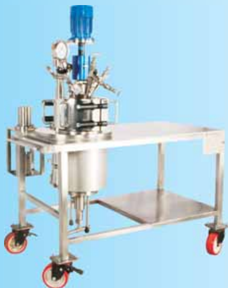
(g) 10 Ltr. autoclave with taper clamp sealing
