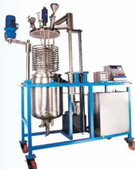
(i) 100 lit autoclave with hydraulic head raising lowering arrangement
