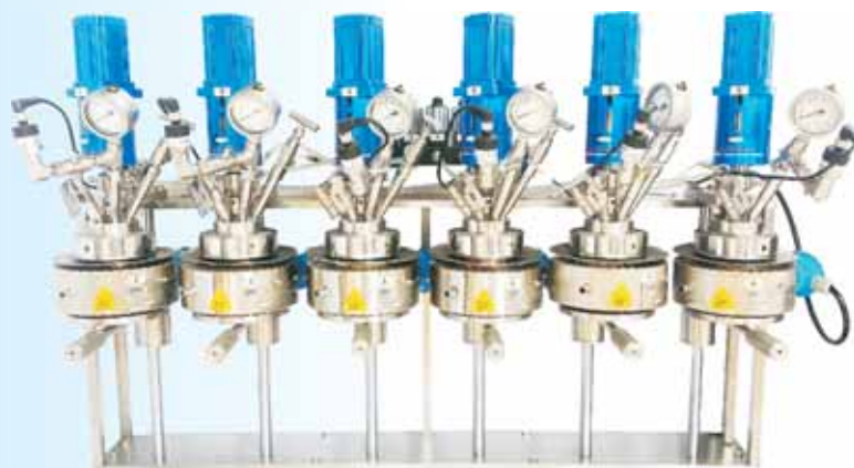
M6 model with fixed head design & inline BLDC motors
