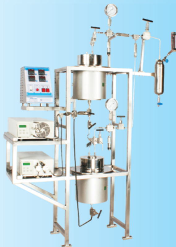
1 ltr. extraction vessels in serial & parallel for 690 bar (10,000 psi) pressure with CO 2 pump
